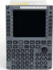
MCDU (MULTIPURPOSE CONTROL DISPLAY UNIT)
